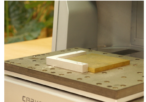
Securing Brass Stock to the bed of the Carvera Air CNC
